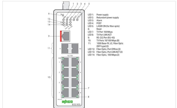
The 852-303 Industrial Switch is a 8-port 10/100Base-TX and 2-port SFP 100Base-FX/1000Base-FX/SX (optional SFP modules) configurable ETHERNET switch.
