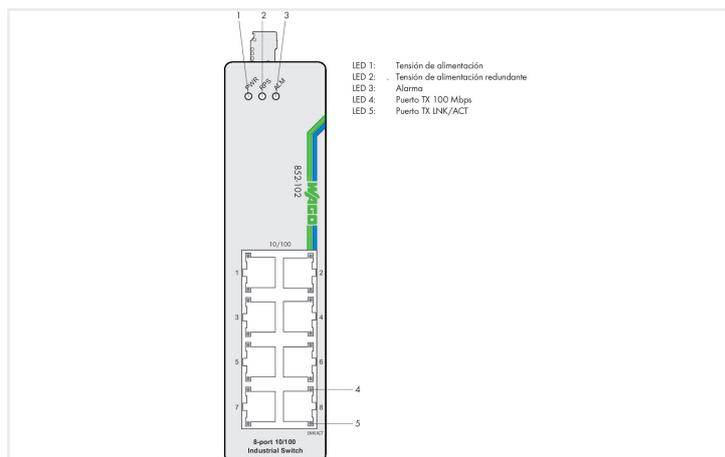
The 852-102 Industrial Switch is a 8-port 10/100Base-TX ETHERNET switch.
