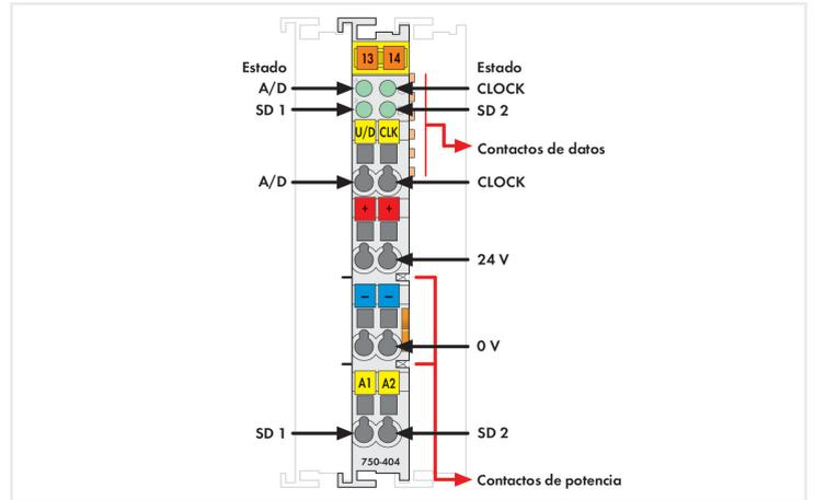
This counter records 24 V binary pulses and transmits the counter status to the fieldbus system. The U/D input allows either Up or Down counting. Digital outputs DO 1 and DO 2 can be set using the control byte. The control byte sets or resets the counter. A counter lock-out is also possible.
