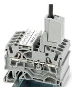
Testing tap (2009-182) for tool-free connection of test cables up to 2.5 mm<sup>2</sup> (12 AWG) – compatible with 2000 to 2016 Series
